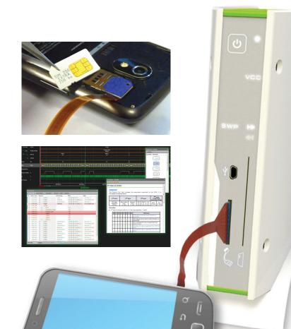
ContactLAB is an advanced laboratory solution designed specifically to address the challenges of validation for contact smart cards and USIM in NFC enabled mobile handsets implementing Single Wire Protocol (SWP) and ISO 7816 interfaces. It encompasses the roles of both a fully programmable laboratory reader, SWP signal emulator and protocol analyzer.
